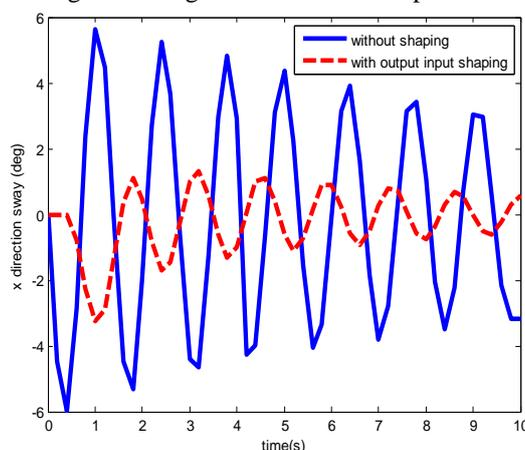
Figure 3. Trolley payload sways
