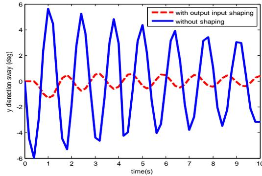
Figure 4. Rail payload sways
